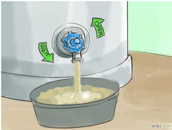
**5. Remove any sediment that has collected at the bottom of the water heater.**
