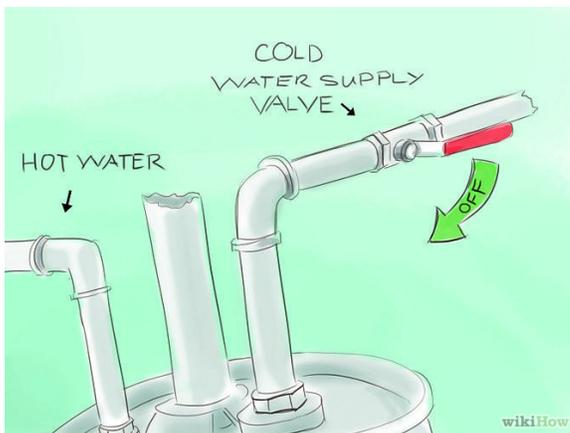
**2. Preserve the cleanliness of the water in the tank by closing the supply valve to the tank.** When water service is restored, the water department will be pumping water that could be contaminated. This will be fine to use for flushing toilets and for cooking, but not for drinking.
