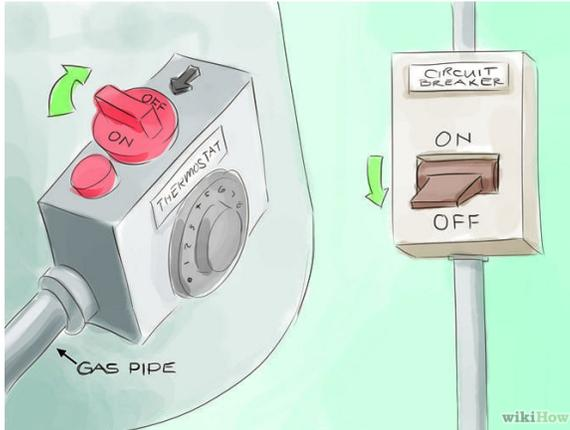
1. **Turn off the electricity or gas to the water heater.** Turn off the circuit breaker for electric water heaters or close the gas valve for natural gas and propane types. If the power is still on when the tank is empty, your tank will almost certainly sustain significant damage. Most electric water heaters in residential applications are 208/240 volts, and supplied by a double-pole circuit breaker or two fuses rated at 30 amps.
